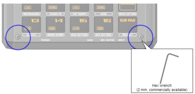
2. Remove the screws (at the far side of the unit) circled in red.
