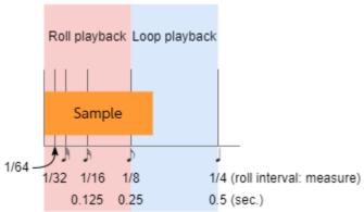
When the roll interval is set to 1/64–1/8, the sample plays back as a roll. When the roll interval is set to 1/4, the sample plays back in a loop.
