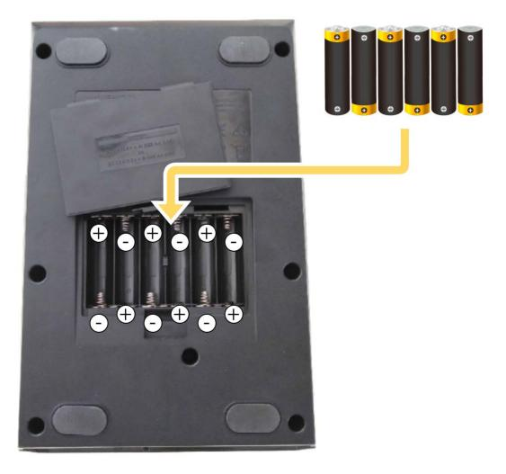
This unit uses six AA batteries (rechargeable Ni-MH or alkaline).
