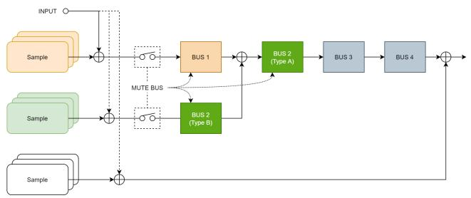
Also, the diagram below shows how the audio outputted from this unit changes when you turn MUTE BUS on/off.
