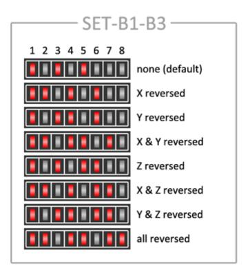
**Acc. orientation:** Allows to swap or shift axes, so you can replace any axis for any other in order to achieve meaningful responses - this may be useful if your unit is a DIY kit in a custom enclosure.
