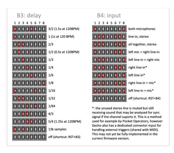
The odd 13k samples delay is there because it is originally used by Dekrispator on STM32F4 platform, it is selected by default when this channel runs (but it can be switched to any other delay, or off - just like in any other channel).
